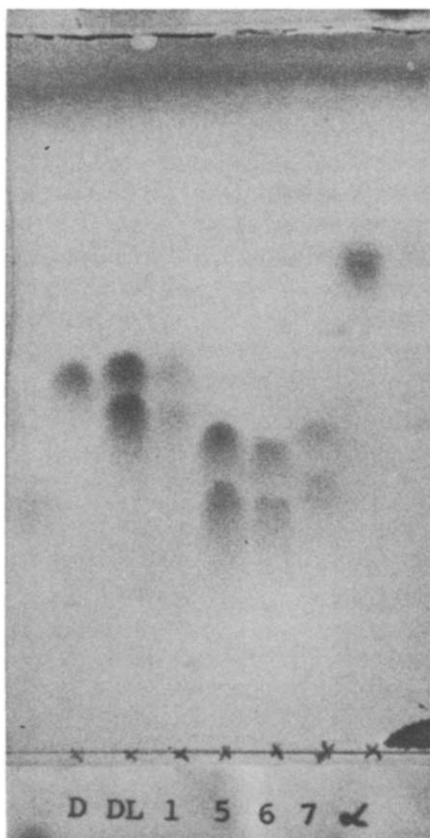
Fig. 1. Chromatogram on a Merck cellulose thin layer developed at room temperature with 0.5 M lithium chloride solution. The spots were revealed with iodine vapour. D = D-tryptophan; DL = DL-tryptophan; 1 = DL-1-methyltryptophan; 5 = DL-5-methyltryptophan; 6 = DL-6-methyltryptophan; 7 = DL-7-methyltryptophan; \alpha = DL- \alpha -methyltryptophan.
